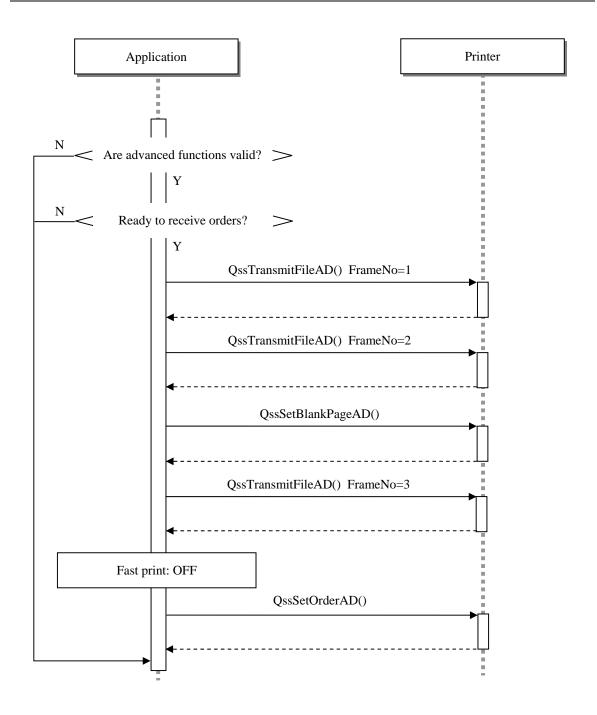
When the fast print function is used: Application Printer Are advanced functions valid? >> Ready to receive orders? Fast print: ON Number of blank pages: 1 QssSetOrderAD() QssTransmitFileAD() FrameNo=1 QssTransmitFileAD() FrameNo=2 QssSetBlankPageAD()  $QssTransmitFileAD()\ FrameNo=3$
